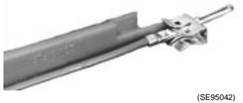
Fig. 10 Lead retention clip details
